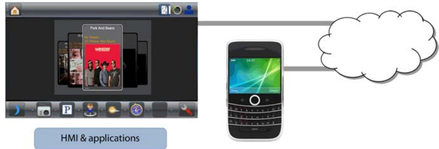
Figure 2: The embedded model connects directly to the cloud and benefits from the more powerful vehicle antennae.
