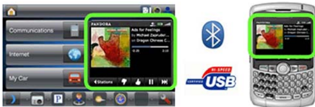
Figure 7: Terminal mode replicates the smartphone HMI on the head unit, which has some control over how and where it is displayed.
