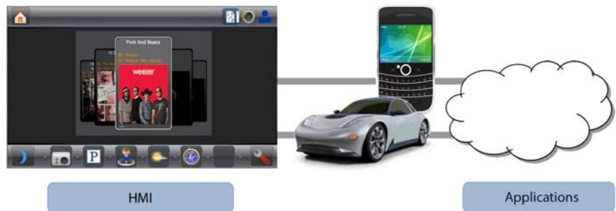
Figure 4: The cloud services model can use the vehicle system and antennae or the smartphone to connect to applications running on remote servers.
